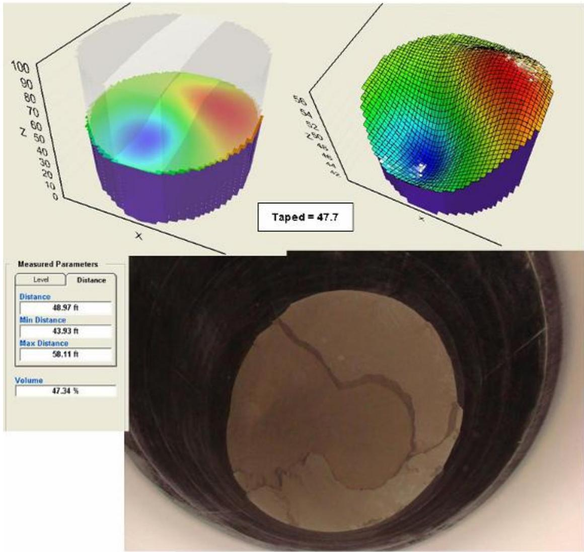
(2) The ability to reach unprecedented volume accuracy. The accuracy reached with the described technology:
