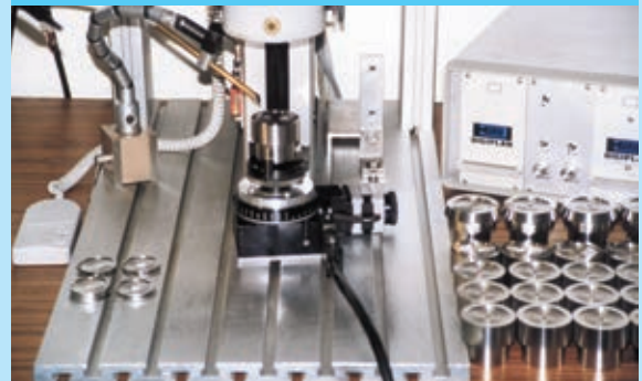
Laser welding of diaphragms.
